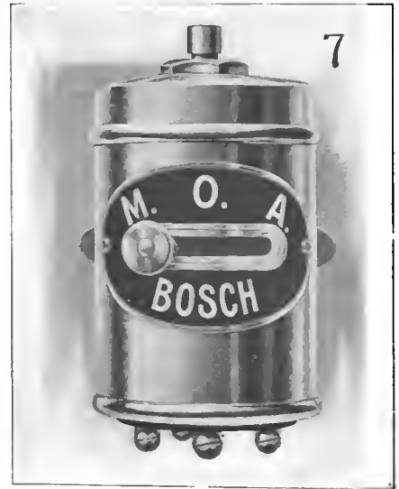
Fig. 7.—Dash Coil and Self-contained Switch.
